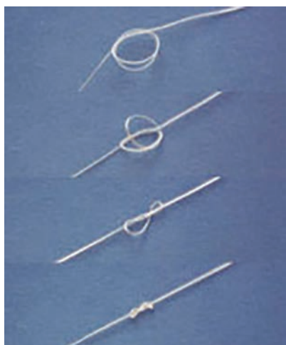
Fig. 7: Tightening of smart suture after raise preparation in thermal temperature
