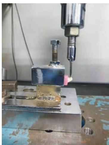
Fig. 9: Application of shear load on universal testing machine
