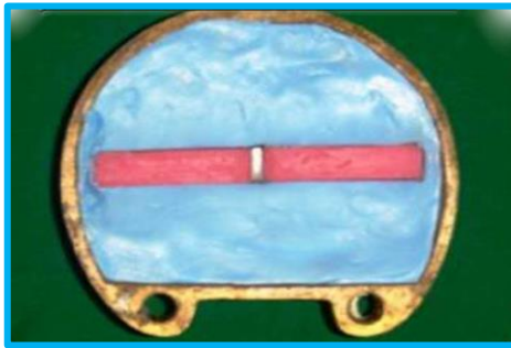
Fig. 3: Acrylic specimen in silicone mold with 3mm metal spacer
