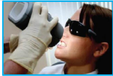
Fig. 2: Use of Optilume TrueShade – which consists of LED lighting to provide a colour corrected light output of 5500K
