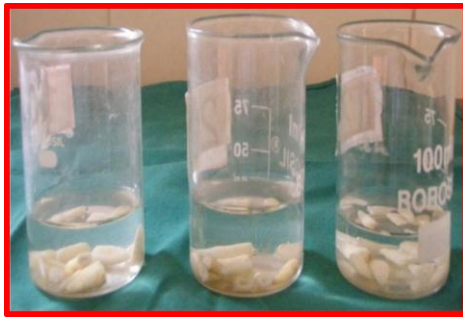
Fig. 1: The samples were left in the irrigation solutions for a period of 15 mins before microbial testing
